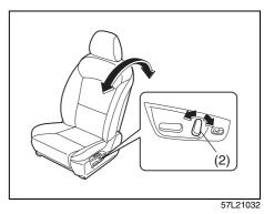
Tilt the reclining switch (2) forward or rearward to adjust the angle of the seatback.
